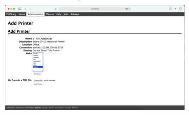
Finally, select Zebra ZPL Label Printer in the Model drop-down list and click Add Printer.
